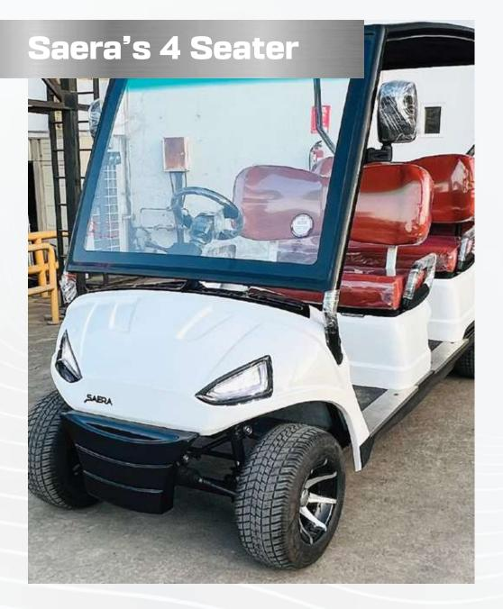
Vehicle model SEAPL 04 48V AC Drive System Seating Capacity 4 person 2850mm Overall Length Overall Width 1225 mm OVERALL HEIGHT(With Sun top) 1870mm 1280mm OVERALL HEIGHT(Without Sun top)
