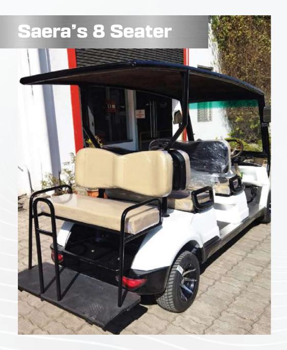
Vehicle model SEAPL 08 48V AC Drive System **Seating Capacity** 8 person 3350mm Overall Length 1225 mm Overall Width OVERALL HEIGHT(With Sun top) 1870mm 1280mm OVERALL HEIGHT(Without Sun top)
